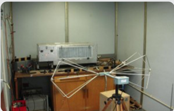
Prototype AC Unit Undergoing EMI/EMC Testing
